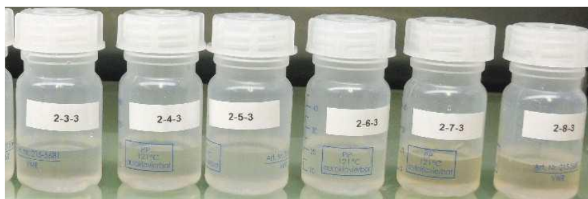
Figure 3. Electrolyte samples showing discolouration – Left to Right, 4N Alumina (99.99%), 3N Alumina (99.9%), Boehmite (99.7%)
