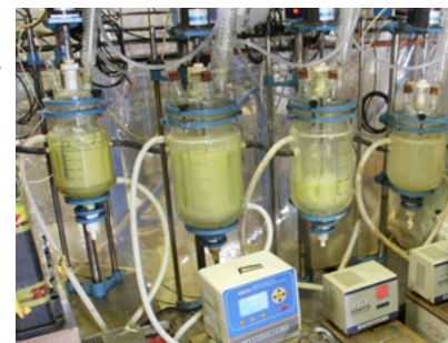
Fig 4. Continuous leaching stage
