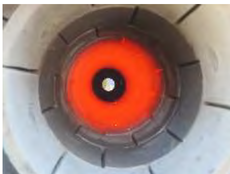
Figure 4. Roaster internal temperature at 700°C
