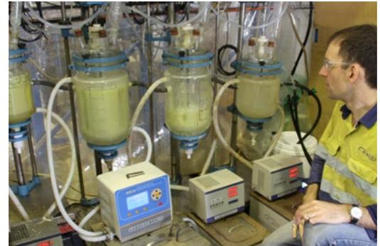
Fig 1. Optimisation test work (continuous leaching test work) is underway on the process flowsheet developed by AMMG
