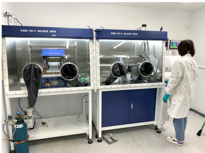
Figure 2 – Pouch Cell Glove Box
